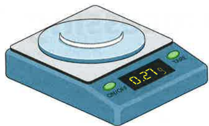
Figure 11.1 This electronic balance reads to two decimal places.
