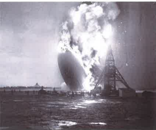
▲ Figure 7.1.8 The Airship Hindenburg accident in 1937 when hydrogen that filled the airship ignited
