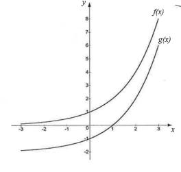
When we add a constant to a function this means that this constant will be added to each value of the function, and the graph will simply be moved up (or down, if the constant is negative) this many steps in the coordinate system. The shape of the curve will be the same.
