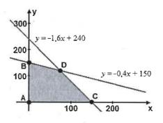
A maximum profit is obtained at point D, that is, if 75 packages of low-grade mixture and 120 packages of high-grade mixture are made. The maximum profit is 510 kr.
