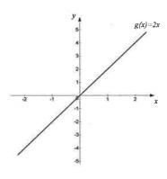
We could now make a guess that if we want to multiply a function by a constant, we can get the new graph by copying the graph of the original function and multiplying the *y*-scale by that constant.
