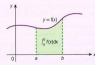
• For a positive continuous function, the area (A) between the graph of the function, the x-axis and the lines x = a and x = b can be approximated by the trapezoidal rule:
