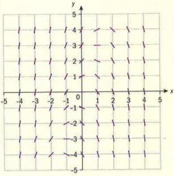
This type of diagram is called a slope field.
